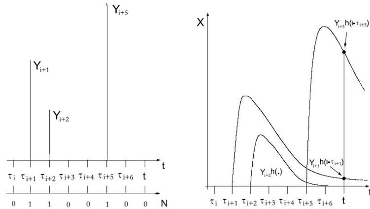
Figure 2 - The graph is an example of the weak influence of remote events (as  $Y_{i+2}$ ) on the runoff formation at time  $t$  (from Giordano, 2004).
