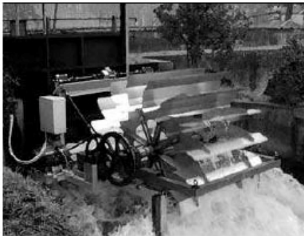
Figure 1. Cross-axis turbine (ENERCAT).
