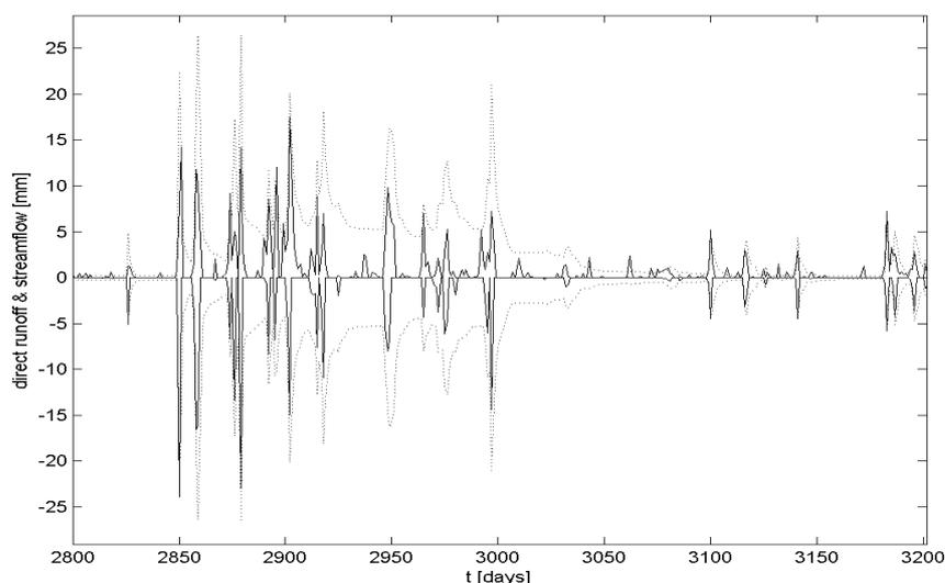
Figure 3. IHACRES (positive axis) and Shot Noise (negative axis) direct runoff, surmounted by the observed (dotted) streamflow for the Scrivia river basin.
