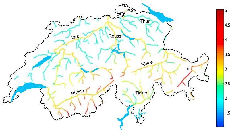
Figure 4. Variability of the return period ratio (referred to the 100-years undisturbed flood, under the hypothesis of \Delta T = 2^{\circ}\text{C} and \Delta\alpha = 10\% ) along the Swiss river network. The names of the main rivers are indicated on the map.
