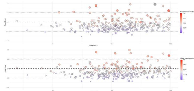
Fig. 2 - Regional model *weighted Nash-Sutcliffe efficiency* (above calibration period 2010 – 2020, below validation period 2000 – 2010)
