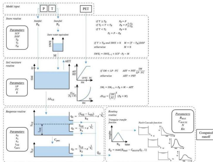
Fig. 1 - Schematic representation of the fully modified *TUWmodel*
