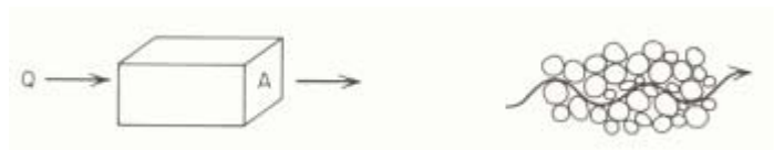
Figure 24. Macroscopic and microscopic concepts of porous medium flow (Freeze/Cherry, Groundwater, © 1979. Electronically reproduced by permission of Pearson Education, Inc., Upper Saddle River, New Jersey).
